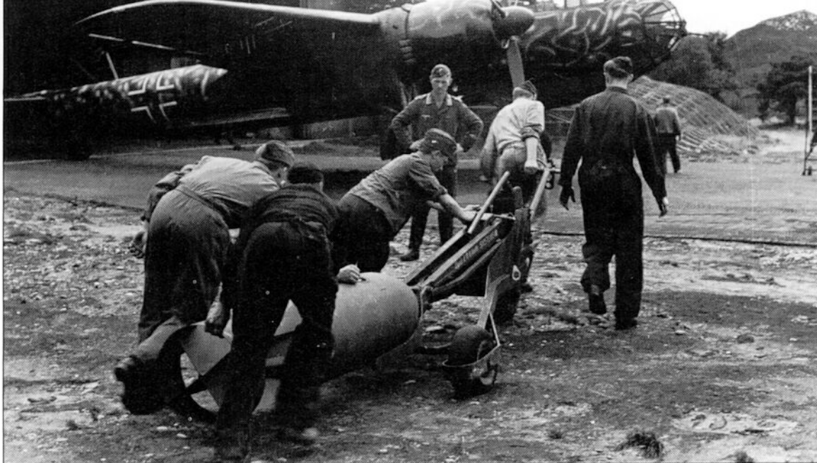
Left: Ground crew manhandle a bomb towards the waiting bay of a Do 217E-1. The aircraft wears a crude Wellenmuster scheme, indicating a primary overwater role. The Do 217E had a long bomb bay which reached from aft of the ventral step to the fuselage cross marking. Normal internal loads consisted of eight 250-kg (551-lb) bombs, four 500-kg (1,102-lb) bombs or a combination of two 1000-kg (2,205-lb) and two 250-kg (551-lb) weapons.
