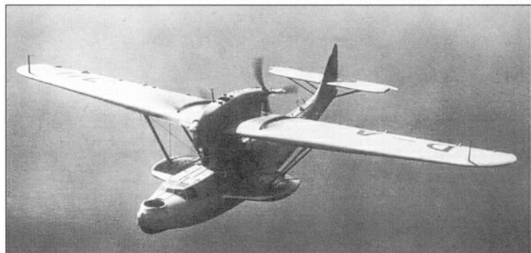
Showing the open bow position to advantage, this aircraft was the pre-production Do 18D-01. The Stümmel sponsons were a Dornier trademark.
