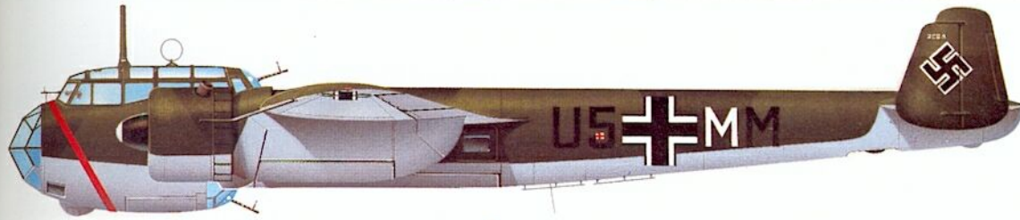
Dornier Do 17Z-2 of 4. Staffel/Kampfgeschwader 2, 1939-40. After service in the Polish campaign, KG 2's next action was over France, where the Do 17Z-2 again proved its ability to outrun fighters in a dive.
