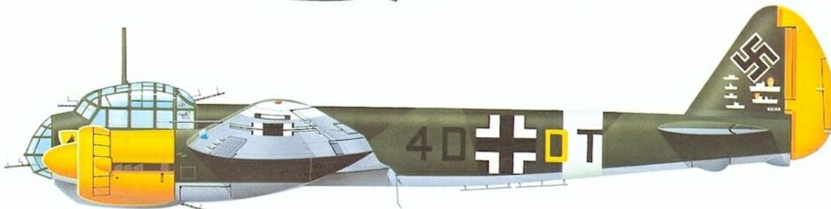
Right: This Ju 88A-5 was used by the III Gruppe of Lehrgeschwader 1 for operations against Malta during early 1941, when the unit was based at Catania, Sicily, as part of Fliegerkorps X. The strengthened landing gear of the A-5 made it more suitable than the A-1 for operations from primitive Sicilian airstrips.
