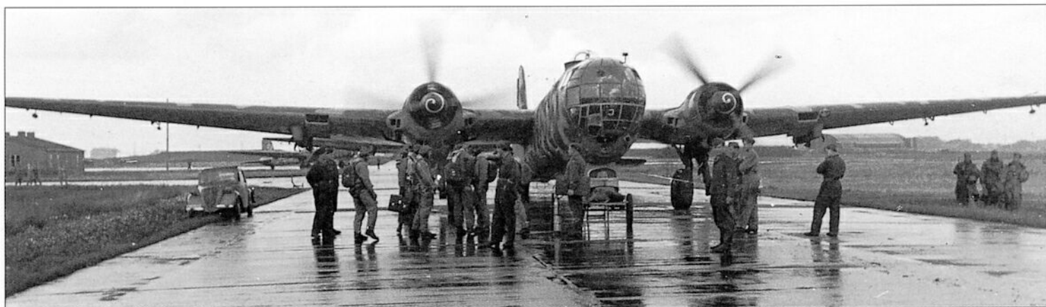
Below: An He 177A-5 of KG 100 rests between missions. Of note is the enormous diameter of the four-bladed propeller, necessary to transmit the power from the coupled engine, and the unique double mainwheel units which retracted outwards and inwards either side of the engine nacelle.
