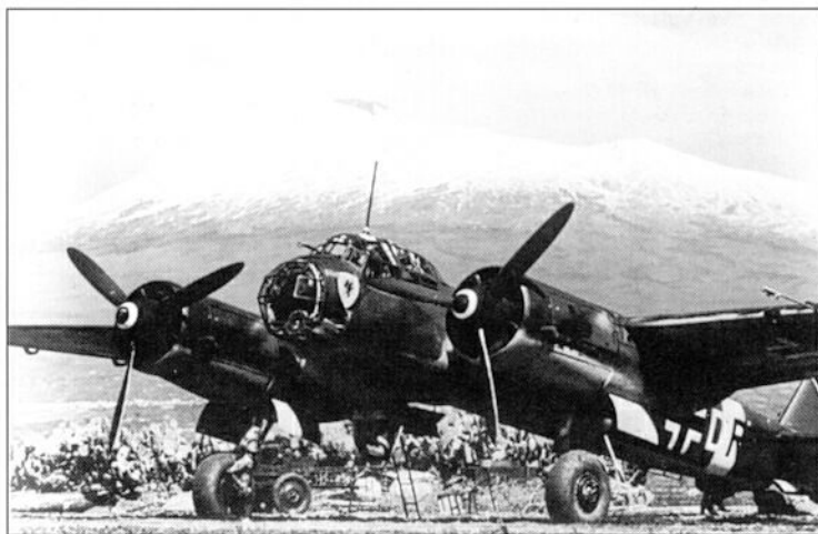
A Ju 88A-5 of III/KG 30. The A-5 was basically a Ju 88A-1 with the long-span wings developed for the up-engined Ju 88A-4, which was delayed by engine problems. It entered service in time for the Battle of Britain.
