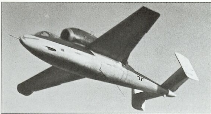
A Heinkel He 162A-1 at speed shows clearly the turned-down wingtips first introduced on the V3 to overcome excessive dihedral problems. The A-1s were manufactured in parallel with prototypes, which themselves were regarded as A-0 pre-production airframes.
