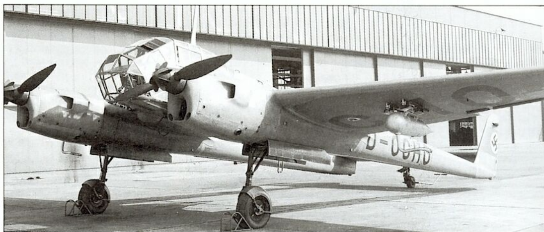
The Fw 189 V4 served as a prototype for the production A-series aircraft, embodying minor changes such as revised cowlings. It later went on to various warfare trials, as seen here with Lost chemical warfare equipment under the wings for the spraying of mustard gas.
