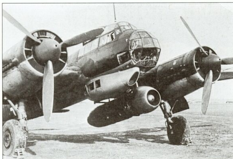
This Ju 88A-5 served as a testbed for the BMW 003 jet engine, powerplant for the Me 262 and Arado 234 jets. As the war progressed, such second-line duties became the lot of early Ju 88 variants.
