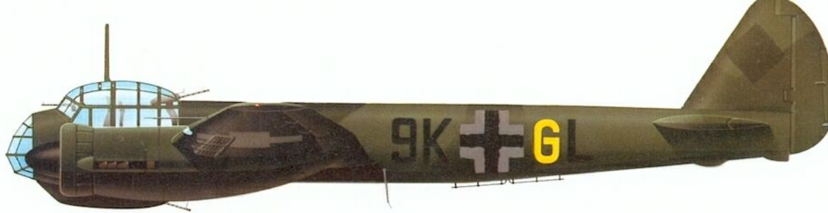
Right: This Ju 88A-5 was used by the III Gruppe of Lehrgeschwader 1 for operations against Malta during early 1941, when the unit was based at Catania, Sicily, as part of Fliegerkorps X. The strengthened landing gear of the A-5 made it more suitable than the A-1 for operations from primitive Sicilian airstrips.
