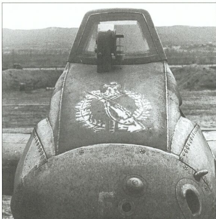
This close-up shows just how cramped the cockpit was, particularly at head-height. Note the infantry-attack badge of the Schlacht units.
