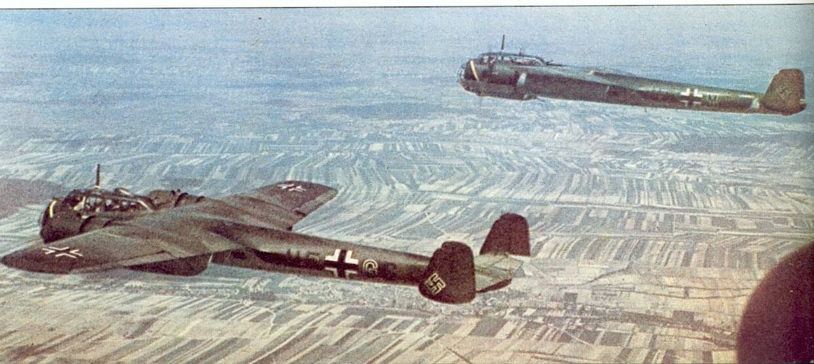
Above: The Do 17P-1 still equipped many reconnaissance units on the outbreak of war, and the similar Do 17M-1 bomber was also on charge. Note the slim fuselage of these early aircraft.
