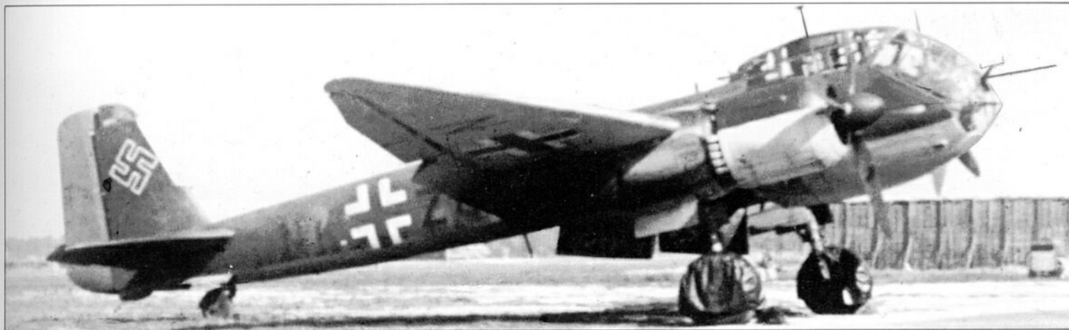
This aircraft at Bordeaux-Mérignac is a Ju 188E-2 with its Hohentwiel radar removed. The EDL 131 turret which normally sat atop the canopy has been removed in favour of a radio aerial.
