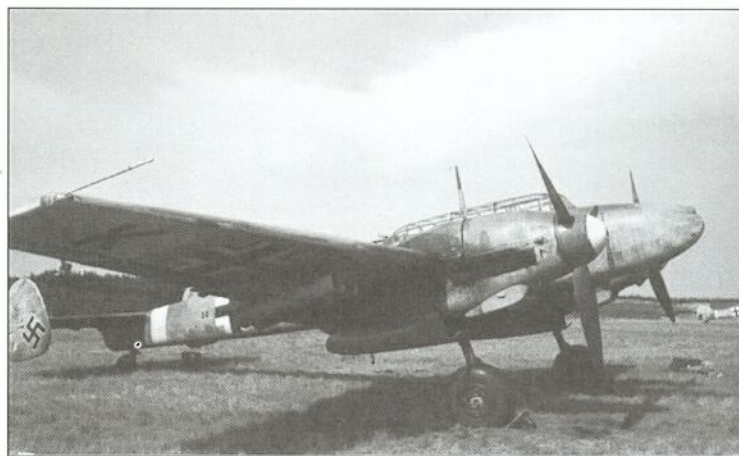
Above: By the summer of 1943, 7./ZG 26 was operating Bf 110G-2/R3s in the home defence role, often armed with underwing Wfr.Gr.21 mortars.
