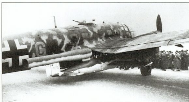
Right: The He 111H-22 was the Fi 103-carrying version, produced by conversion of incomplete H-21s on the production line or from existing H-16s and H-20s. This example served with 1./KG 3 at Venlo in the Netherlands.
