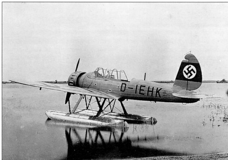
This view of the prototype Ar 196 shows the twin-float layout that became the standard. The horn balance on the rudder was discarded for the V2, which was similar apart from this and changes to the water rudders. Both aircraft flew in the summer of 1937.
