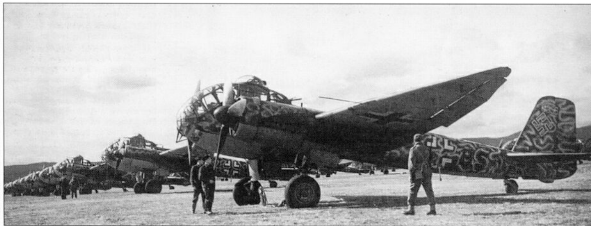
Left: A line-up of Ju 188D-2s of 1.(F)/FAGr 124 at Kirkenes, Norway. The Ju 188D-2 was intended primarily for the maritime strike and reconnaissance role, and most had FuG 200 Hohentwiel radar.
