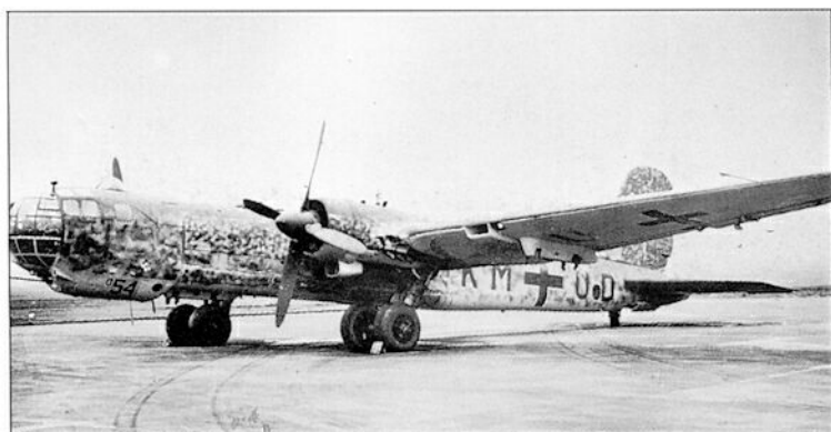
6. Staffel of Kampfgeschwader 100 was based at Toulouse-Blagnac during May 1944, using its He 177A-5s on bombing missions. This He 177A-5/R2 still has factory codes applied prior to delivery. Note the underwing and ventral racks for Hs 293 missiles and Fritz X guided bombs.
