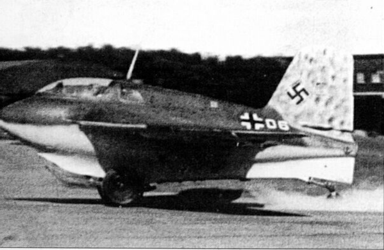
An Me 163B (actually the Bertha prototype) makes a 'sharp start' at Bad Zwischenahn, home of the trials unit Erprobungskommando 16, which accepted its first Me 163B during May 1944. The jettisonable take-off trolley is clearly visible.
