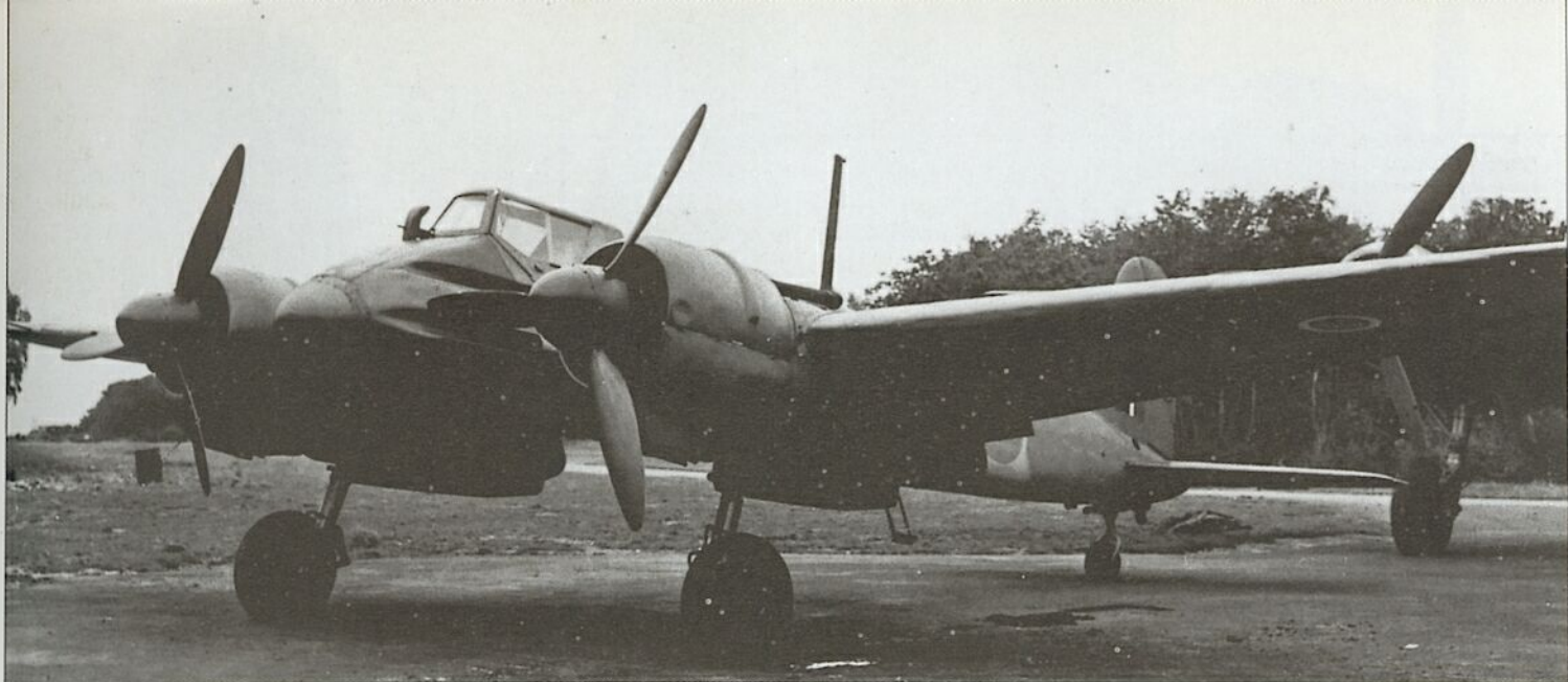
This Hs 129B-1 is seen in RAF colours after capture. On either side of the nose were mounted MG 17 7.9-mm (0.31-in) machine-gun (lower) and a MG 151 20-mm cannon (upper). The machine-gun had 500 rounds per gun in the fuselage, while the cannon had only 125.
