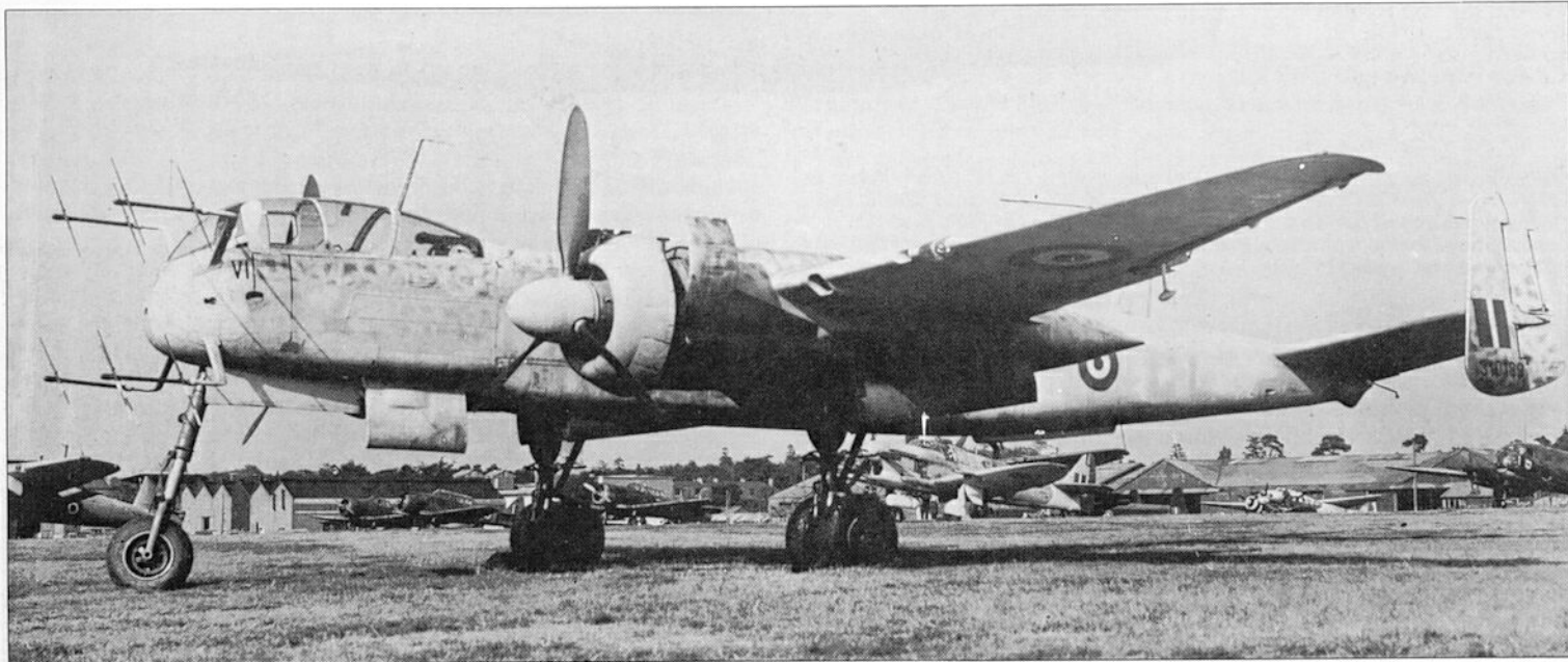
Photographed during evaluation in Britain after the war, this He 219A-5/R2 shows the aft cockpit canopy redesigned to eliminate the provision for an aft-firing MG 131 machine-gun – a feature discarded earlier by most He 219s in operational use.
