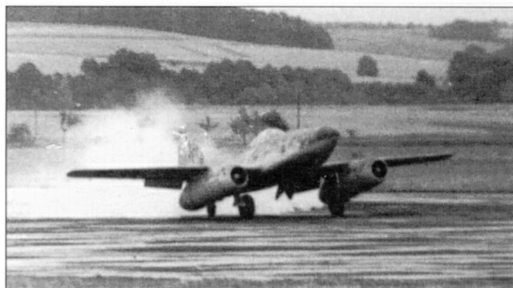
The Me 262 V3 lands after its first flight at Leipheim on 18 July 1942. The smoke was caused by unburned fuel igniting in the jet pipes as it dripped out onto the runway. This was the first flight of the Me 262 using turbojet power alone, the first prototype having also had a nose-mounted piston engine.
