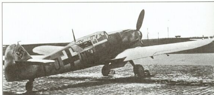
Above: This Bf 109G-12 trainer was converted from a Bf 109G-6 airframe, others being based on randomly selected Bf 109G-2s and Bf 109G-4s. Less than 100 two-seaters were built, of a planned total of over 900 trainer variants.
