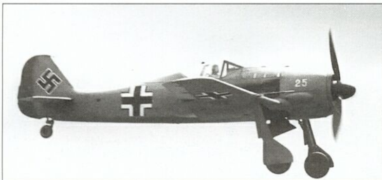
The last of eighteen pre-production Fw 190A-0s on approach. This was the 25th Fw 190 built, and had the full-standard big wing. The first nine Fw 190A-0s had the original narrow-chord wing of the prototype, with greater taper on leading and trailing edges.
