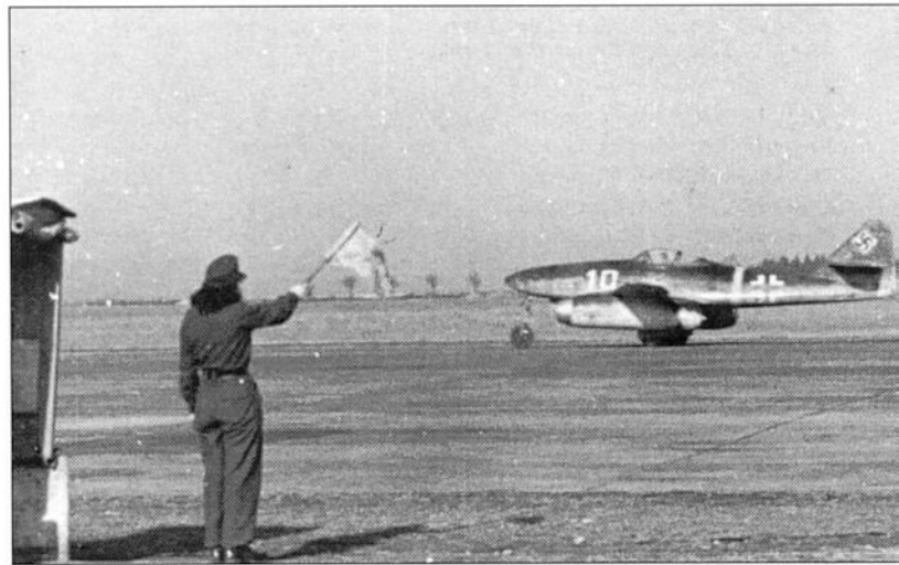
Above: A female Luftwaffe auxiliary signals to the pilot of an EKdo 262 or EJG-2 Me 262A-1a. In the intercept role, the Me 262 could carry 24 underwing R4M rockets in addition to its built-in armament of four 30-mm MK 108 cannon. The aircraft had 100 rounds for each of the upper guns, and 80 for each of the lower pair.
