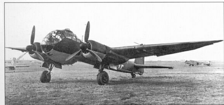
This is the first production Ju 188E-1, which beat the Ju 188A into service because of the readier supply of BMW 801 engines which powered it. The aircraft had a 13-mm machine-gun in the dorsal turret, instead of a 20-mm cannon.
