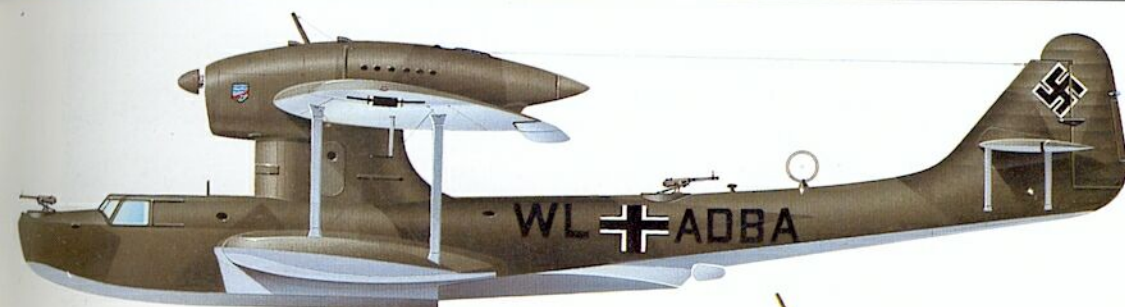
This Do 18D served with Flugzeugführerschule (See) in the summer of 1939. This was a training school for reconnaissance seaplanes. Note the two open positions for the light defensive armament.
