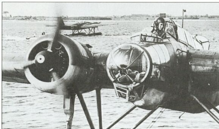
A close-up of an He 115B shows the extensive glazing in the nose area. The bombardier had flat-pane windows in the bottom of the nose for accurate aiming, and it was his duty to fire the nose-mounted MG 15.
