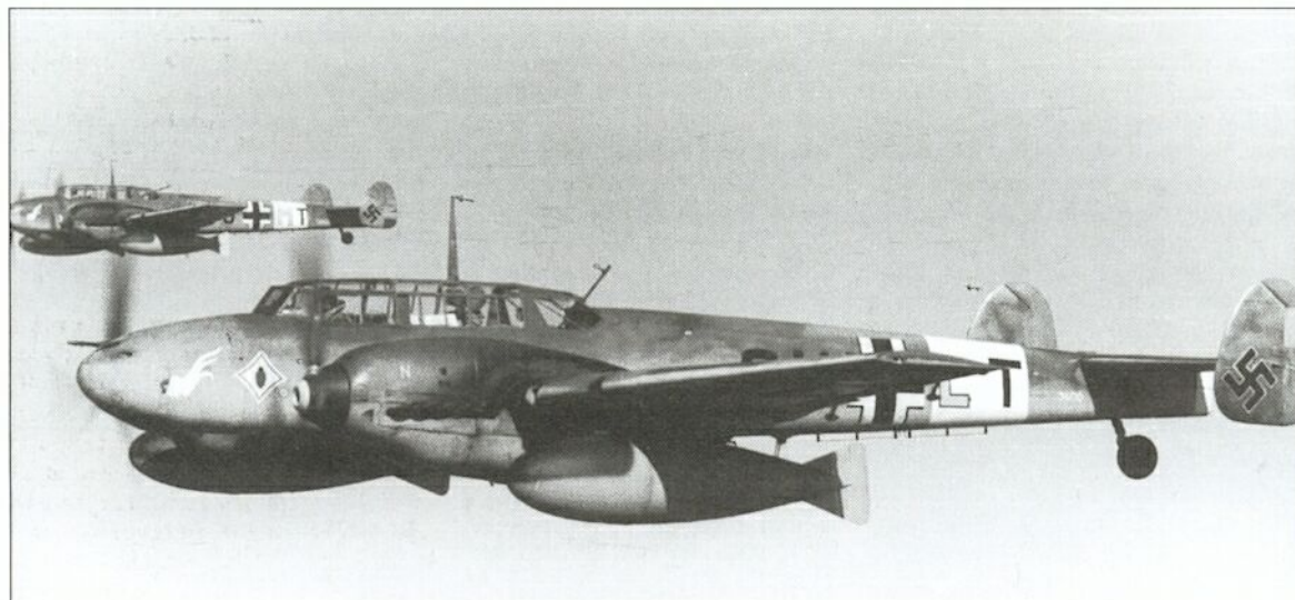
Left: A pair of Bf 110D-3s of 9./Zerstörergeschwader 26 flies over the Mediterranean during 1941, carrying a pair of 900-litre (198-imp gal) fuel tanks for extended endurance in the convoy protection role. The Bf 110D-3 was specifically tailored for the convoy protection role, and carried an underfuselage auxiliary oil tank, with provision for 300- or 900-litre (66- or 198-imp gal) auxiliary fuel tanks under the outer wings. The tailcone was extended to house a dinghy.
