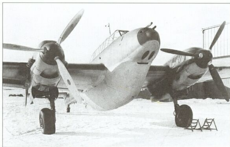
Below: During the day, the night-fighter Messerschmitts hid from Allied bombers under elaborate camouflages involving nets and foliage. This aircraft has the Rustsatz-3 applied, which replaced four forward-firing MG 17 guns with two Mk 108 30-mm cannon.
