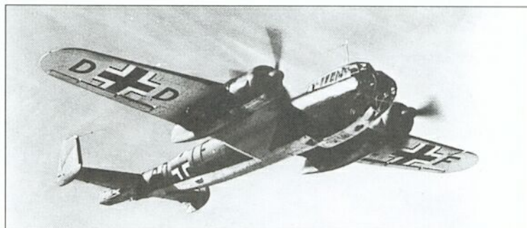
A complete reworking of the basic design introduced the Do 217E, with a much deeper fuselage to allow the carriage of large bomb loads. This aircraft is the sixth pre-production Do 217E-0.
