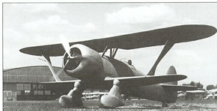
The first prototype Hs 123 featured a smooth NACA-style cowl. It flew in early 1935 and demonstrated excellent performance.
