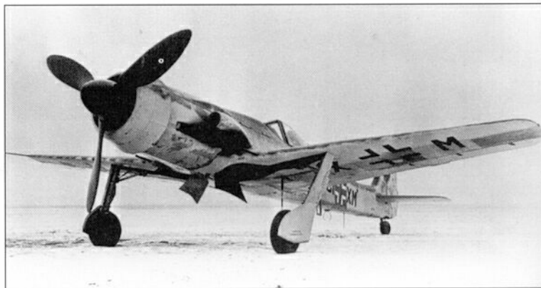
Intended primarily as a Zerstörer, the Ta 152C series featured short-span wings and the Daimler-Benz DB 603 engine, a big improvement in terms of power over the Jumo 213. This aircraft is the V7 prototype, otherwise known as the Ta 152C-0/R11 and featuring Rustsätze bad-weather equipment and an MW 50-boosted DB 603EM engine.
