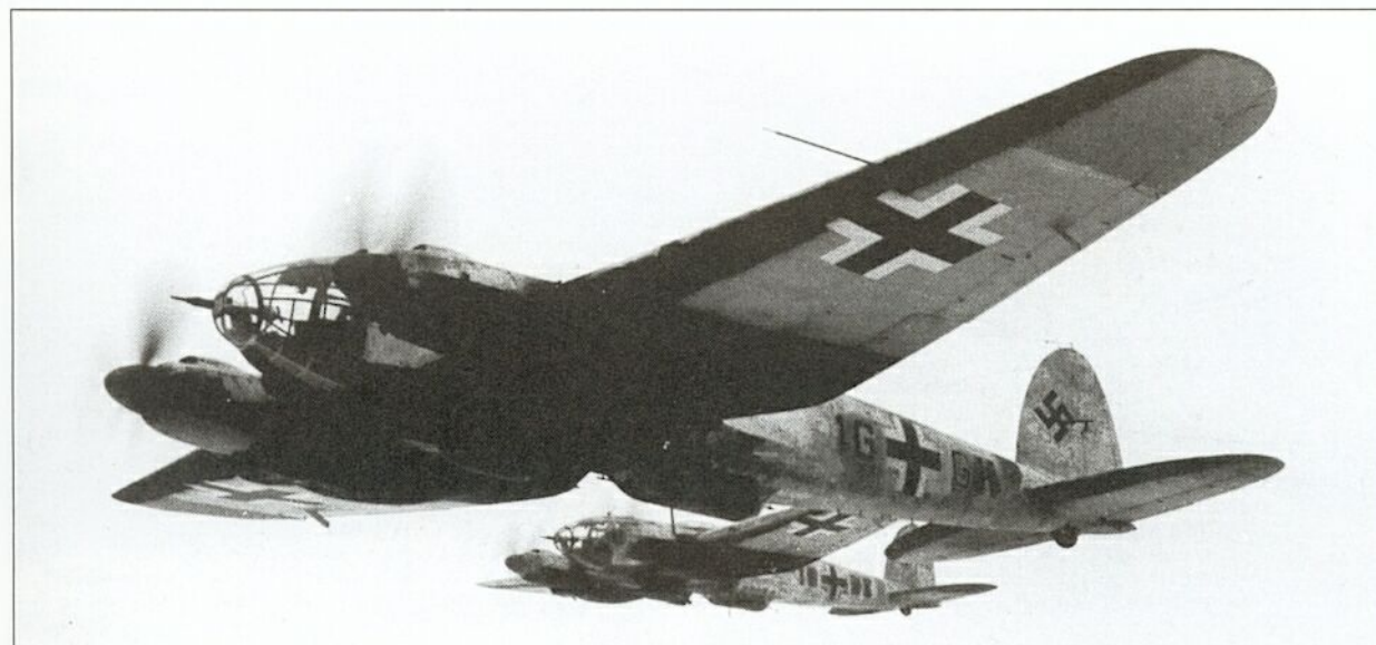
Above: Displaying the soluble white distemper applied for winter operations over the standard camouflage, this He 111H-10 served with 5./KG 4 on the Eastern Front.
