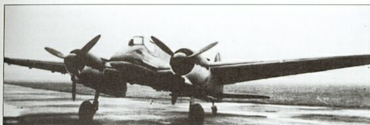
This is the second Hs 129B-0, the pre-production aircraft being distinguished by having the gun blast troughs faired over.
