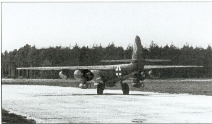
Fitted with Rauchgeräte take-off booster rockets and carrying an SC 500J 500-kg bomb under the centre fuselage and under each engine nacelle, the 10th prototype begins its take-off run. The type began flying operationally in the summer of 1944.
