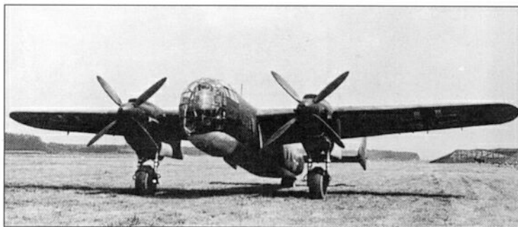
The Do 317 was an advanced extension of the Do 17/217 line, featuring a pressurised cabin. No real increase in performance over the Do 217P was found and, apart from the Do 317 V1 (illustrated), the other five prototypes were completed without pressurisation and used by KG 100.
