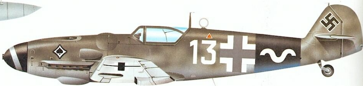
The Bf 109G-14 with 'Galland hood' was a fighter-bomber version of the G-6, this 'Gustav' bearing the markings of III./JG 53. The Spiralschnauze has no significance in this instance. Note the bulges over the breech blocks of the nose-mounted 13-mm (0.51-in) MG 131 guns.
