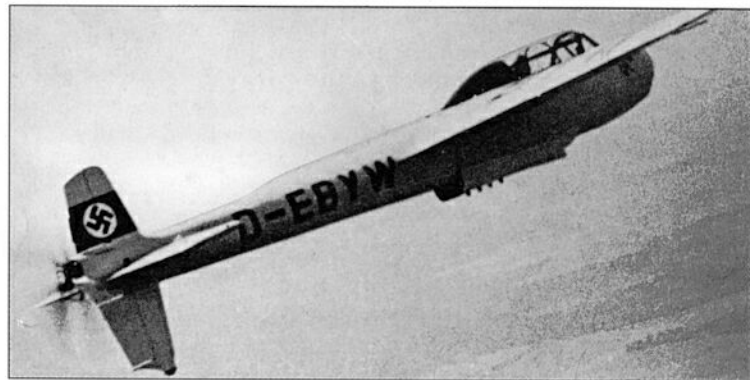
Designed by Ulrich Hutter, the all-wooden Göppingen Go 9 was the testbed for the Do 335's aft-mounted prop design. Built by Schempp-Hirth and powered by a Hirth HM 60R engine mounted below the wing, the Go 9 attained a speed of 220 km/h (137 mph).
