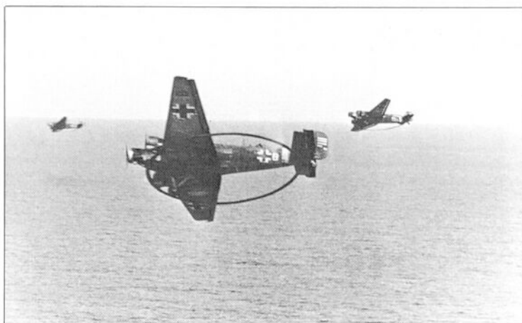
Three Junkers Ju 52/3mg6 mine-clearance aircraft of the Minensuchgruppe, probably over the Mediterranean. The rudder markings are said to have denoted the number of minesweeping sorties flown – a somewhat hazardous task.
