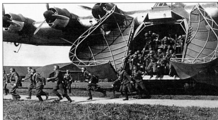
Luftwaffe troops deplane from an Me 323D-1 during evaluation of the type in the air assault role. The Me 323D-1 was built from the start as a powered aircraft, and introduced two nose gun positions, two dorsal gun positions and a reduced number of cabin windows.
