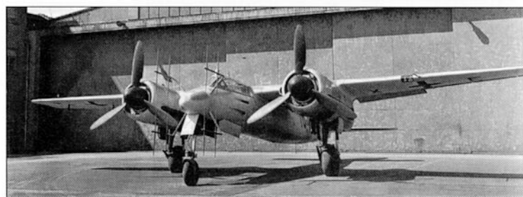
The Ta 154A-0 V15 was the last pre-production aircraft, and featured Hirschgeweih antennas for Lichtenstein SN-2 radar.
