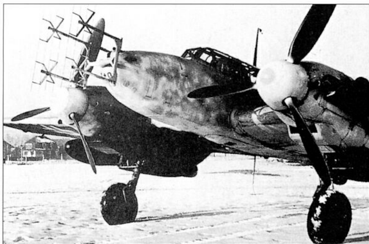
Left: A close-up of this 6./NJG 6 aircraft shows the antennas for the FuG 202 Lichtenstein B/C radar and flame-damped exhaust. The underwing tanks held extra fuel, the fitment of them covered under the designation B2. This example force-landed in Switzerland after becoming lost.
