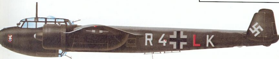
This Do 215B-5 Kauz III served with Stab II/NJG 2 based at Leeuwarden in the summer of 1942, and was the personal mount of Gruppenkommandeur Helmut Lent. It has FuG 202 Lichtenstein BC radar fitted and a ventral tray with MG FF cannon.
