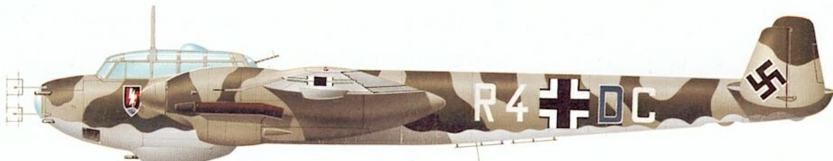
This Do 215B-5 Kauz III served with Stab II/NJG 2 based at Leeuwarden in the summer of 1942, and was the personal mount of Gruppenkommandeur Helmut Lent. It has FuG 202 Lichtenstein BC radar fitted and a ventral tray with MG FF cannon.
