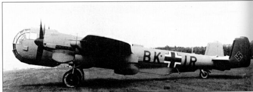
The strange Do 217P V1 (illustrated) featured a DB 605T engine in the fuselage that supercharged the wing-mounted engines. Combined with the pressurised cabin, this gave the Do 217P a ceiling of 16150 m (53,000 ft) in its pre-production Do 217P-0 form.
