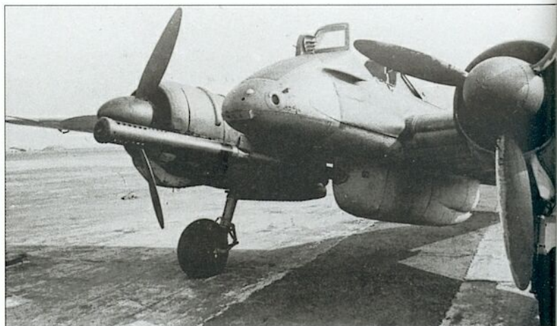
In order to provide a hard-hitting weapon against Soviet tanks, the Hs 129B-3/Wa was evolved, with a 75-mm Panzerabwehrkanone 40 in a large ventral fairing. Performance and agility were drastically reduced, although one shot could knock out the biggest Soviet tank.
