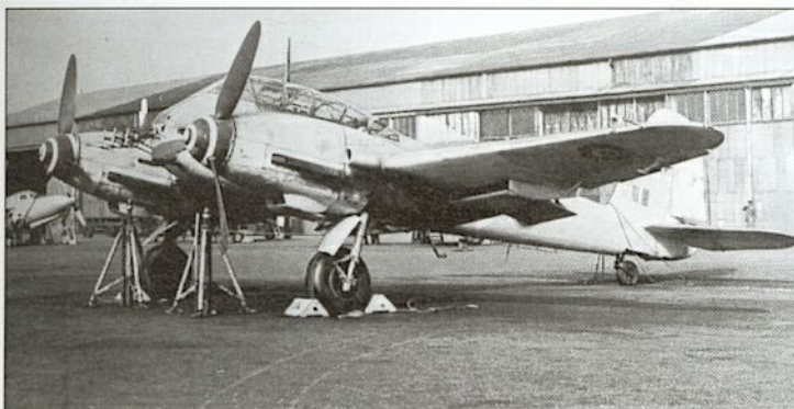
Above: Festooned with nose-mounted antennas for the FuG 200 Hohenzweielf radar, this former I/ZG 1 Me 410B-6 was used in the anti-shipping role, operating from Lorient, before the unit was withdrawn to Germany for air defence duties. Spiral painted spinners were a regular feature of the Me 410.
