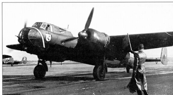
Above: A marshall waves out a III/KG 2 Do 217E-4 for a mission. Visible in the nose glazing is the MG 15 operated by the navigator/bombardier, and below the glazing is the barrel for the fixed MG 151/15 cannon, aimed by the pilot. Do 217s intended primarily for the anti-shipping mission had this latter weapon replaced by a 20-mm MG FF.
