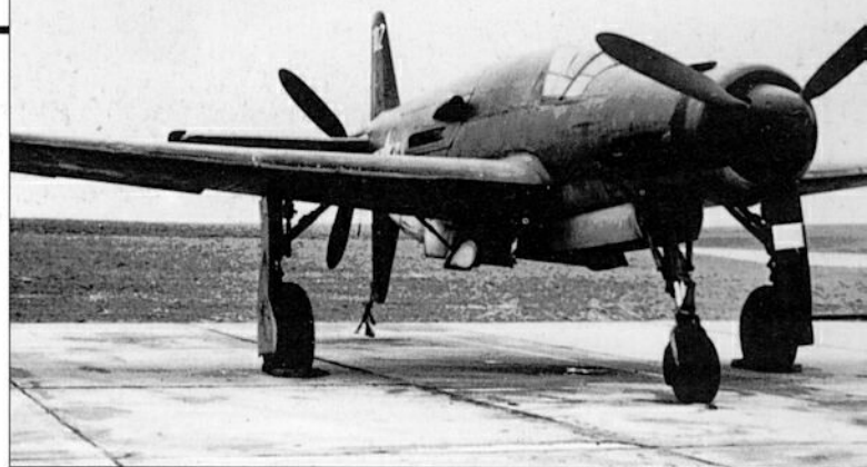
The nose-mounted Daimler-Benz DB 603A-2 engine was provided with an annular nose radiator, while the ventral scoop intake was for the aft powerplant. The tractor propeller was pitch-reversible.
