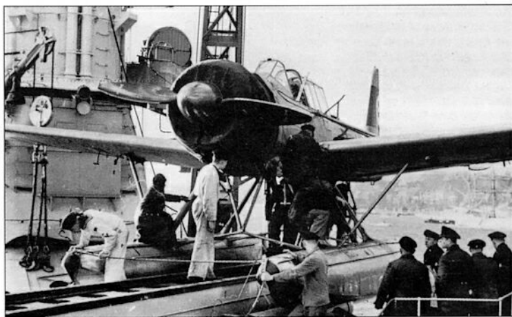
The Ar 196 was designed to meet a requirement to replace floatplanes aboard large ships of the Kriegsmarine. Here one of the prototypes is tested aboard a ship. In operation the aircraft was catapulted into the air for take-off, and hoisted back on board the ship after a sortie.
