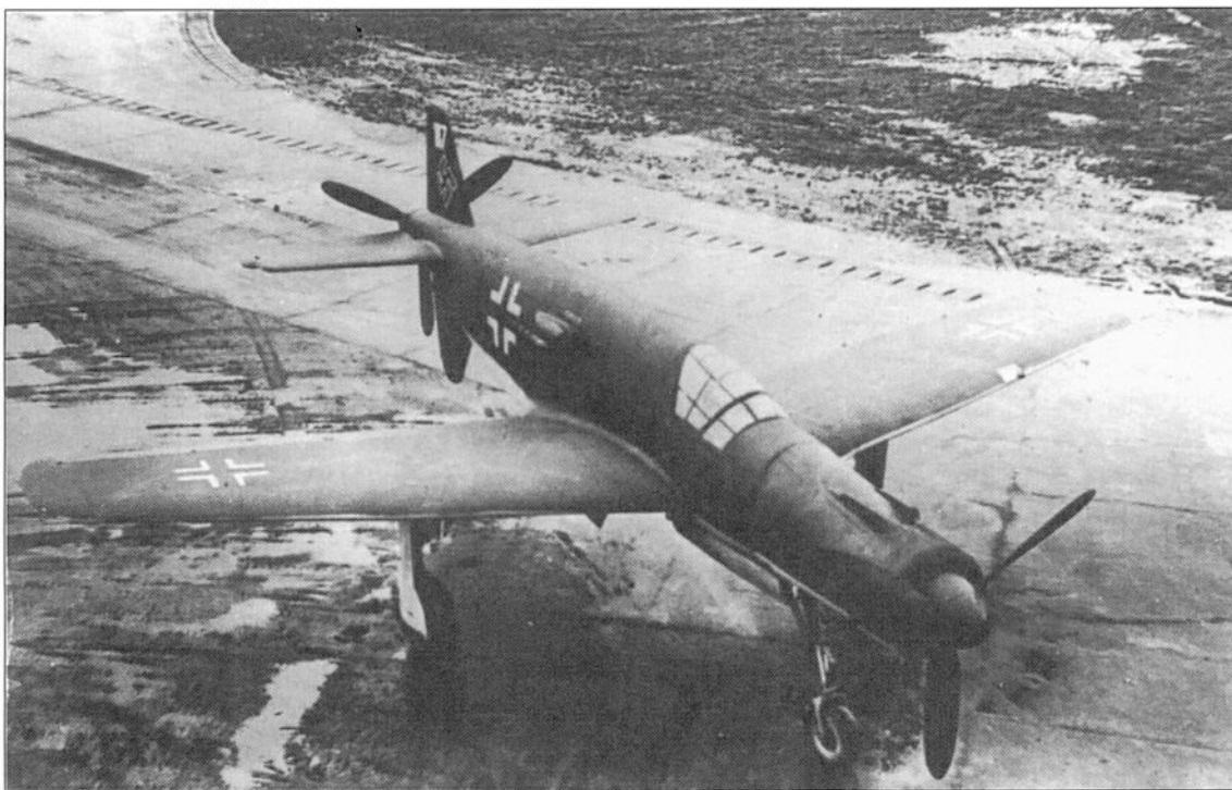
Left: The ten Do 335A-0s (this is the seventh) were intended for evaluation as single-seat fighter bombers and were used by the Erprobungskommando 335 formed in September 1944. The aircraft had full cannon and machine gun armament, and an internal weapons bay. The Do 335A-0 differed from the production model in having two DB 603A-2 engines and lacked underwing hardpoints.
