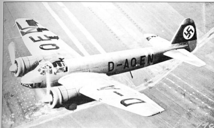
Stooks of corn in the field below are hard to explain in this picture of the Ju 88 V1 (first prototype), because its flying career extended only from December 1936 until the following spring. Note the swivelling cine camera in the position reserved for the upper rear gun, and the separate oil coolers under the DB 600s.
